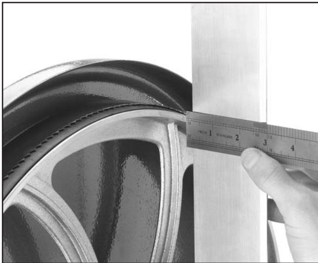
Figure 38. Measuring wheel difference.
